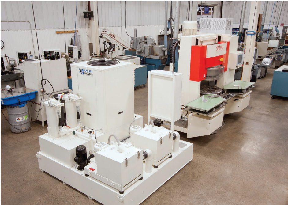
A new Stahli DLM-705 double-disk grinder has the capability to grind at rates 10 times faster than manual machines.
