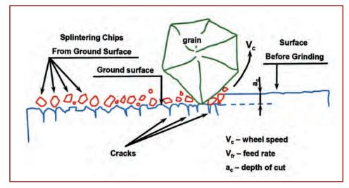
Figure 1. Material removal mechanism.
