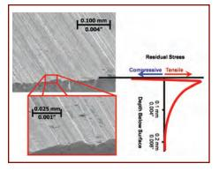
*Figure 2.* A brittle material does not follow the ductile material stress profile.
