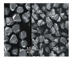
*Figure 3.* Blocky (left) vs. angular-shaped grains.
